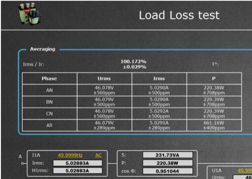
Figure 7 – live accuracy and printout of uncertainty in modern measurement system
