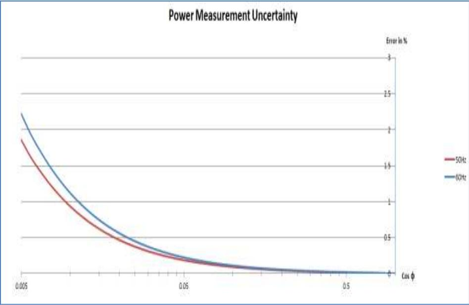
Figure 3 – Power measurement uncertainty in relation to the power factor
