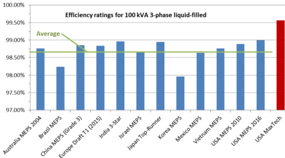
Figure 2 – Efficiency criteria at 50% load for 100kVA liquid filled transformers in different countries<sup>4</sup>
