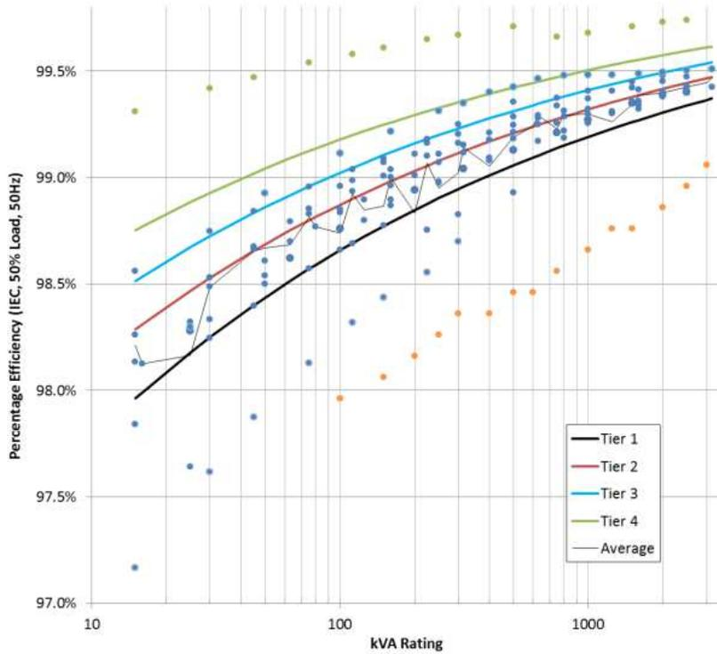
Figure 1 – Liquid filled Transformer tiers – efficiency values<sup>3</sup>
